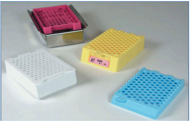
Figure 3. Large format cassettes showing standard (white), slim (blue), and mothership style (yellow). SM mothership mold with SM mothership cassette (bright pink) is in the background.
