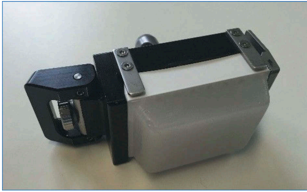
Figure 16. Longer replacement support plates for the Microm adjustable universal macro-cassette clamp. Note the silver arms shown on top of the clamp holding the SM cassette with paraffin block. These arms on the longer plate provide improved stability for SM blocks during sectioning when the clamp is in the horizontal position as shown.
