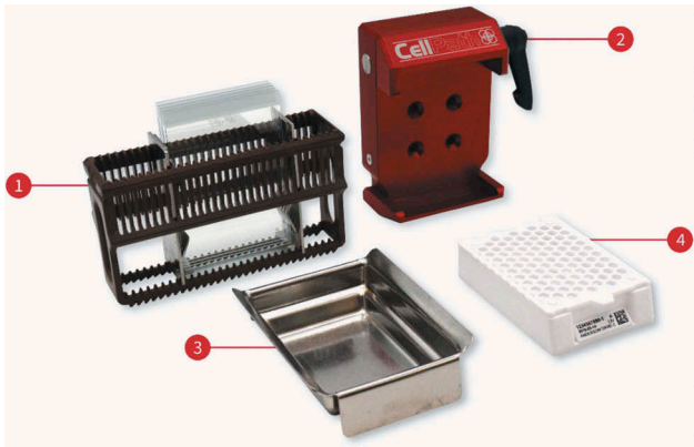
Figure 1. Essentials required for setting up large format include [1] slides and staining rack with adapters [2], cassette clamp [3], embedding molds and [4] processing cassettes.
